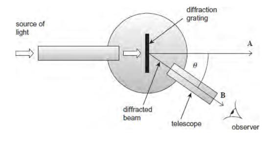
(b) (i) When the spectrometer telescope is rotated from an initial angle of zero degrees, a spectrum is not observed until the angle of diffraction  $\theta$  is about 50°. State the order of this spectrum.
